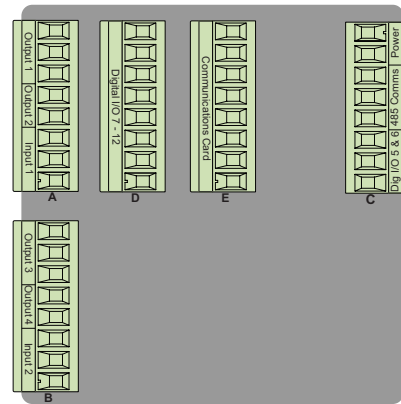
Back View Slot Orientation 1/4 DIN Horizontal PM4
