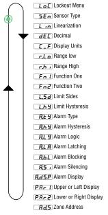
**Setup Menu** 16<sup>th</sup> & 32<sup>nd</sup> DIN Limit Controller Range Parameter Name Description Display Defaults are shown **bold** Alarm High Set Point
