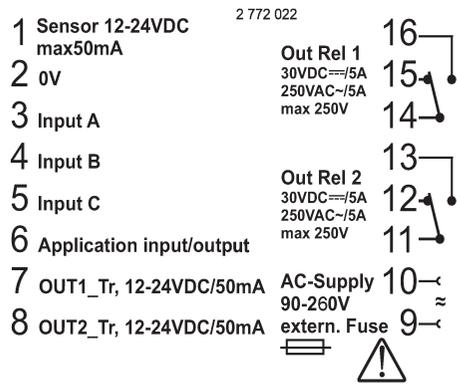
VAC switching power supply 2 relays / 2 transistors
