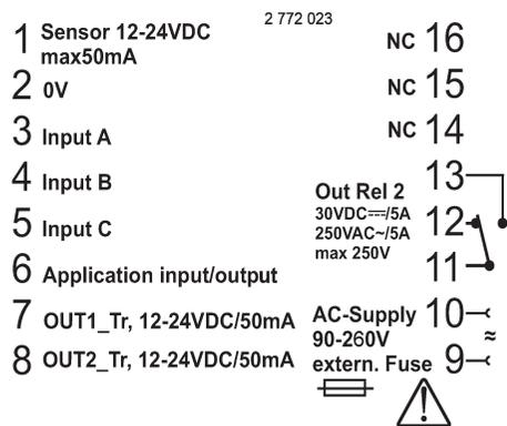
VAC switching power supply 1 relay / 2 transistors
