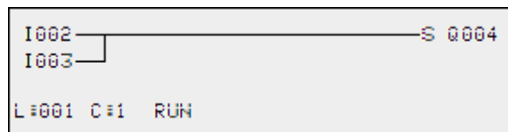
Figure 90: Power flow display
